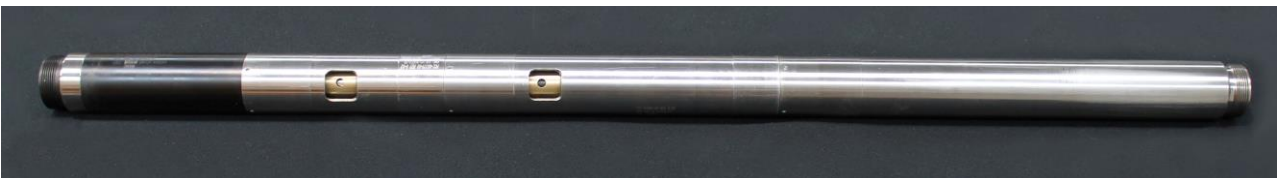
Valve API 14A V3 Annex B Qualified at SwRI.
